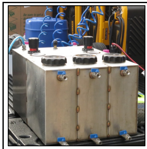
Figure 1. Dry-fog application system.
